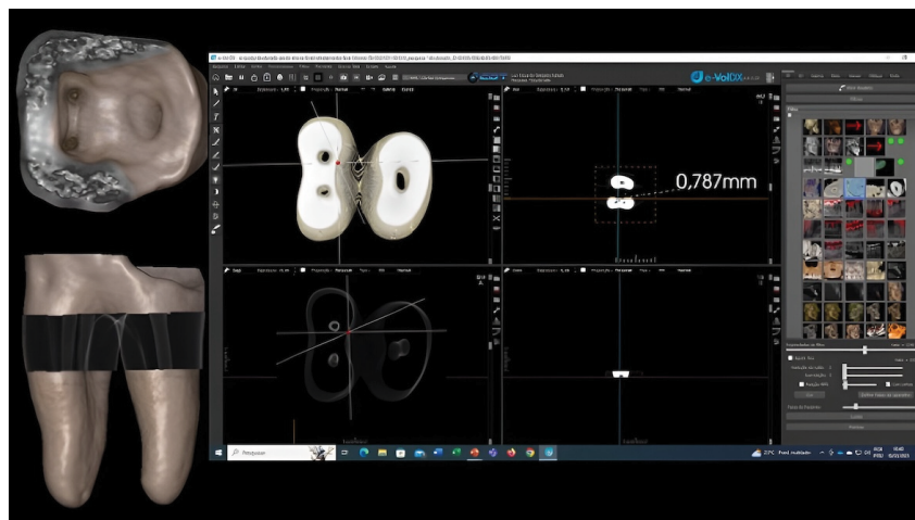
Figure 2. Illustration showing the synchronization of the 2D mode adjusted to have the same dimension as the 3D image. Dimensions were calibrated until the 3D and 2D modes matched.
