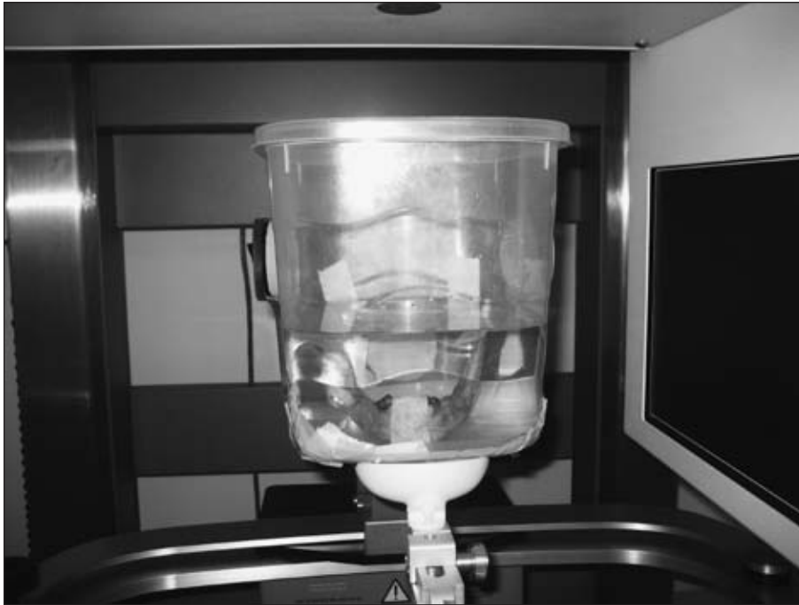
Figure 1 - Container with water and the mandible simulating patient position in the i-Cat Vision® device for CBCT acquisition.
