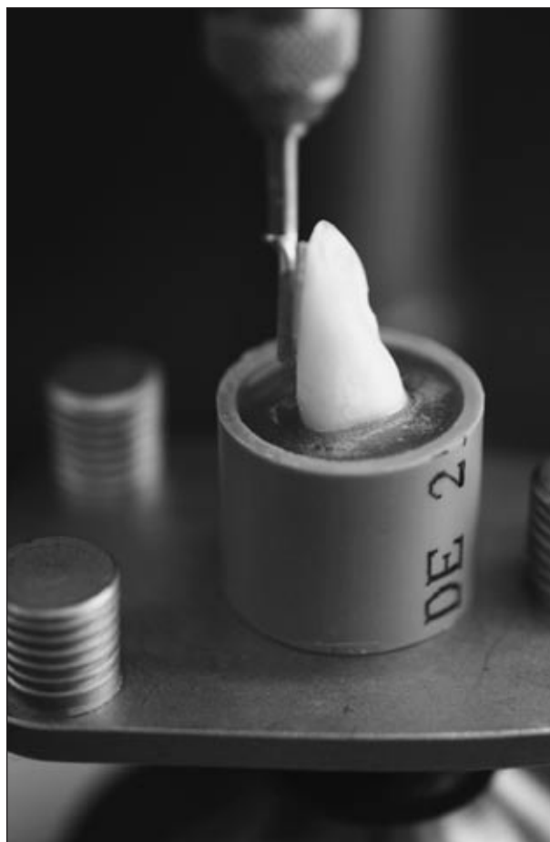
Figure 2 - Use of the surveyor (Bio Art) to prepare the test specimens.
