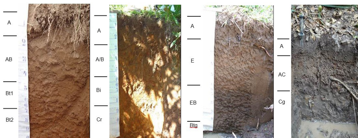
Figure 2: Looking from left to right, profile image of the Ultic Hapludalf (P1), Oxic Dystrudept (P2), Oxyaquic Hapludalf (P3) and Humaqueptic Endoaquent (P4), showing the variation of solum depth (depth of A and B horizons) related to soil development.
