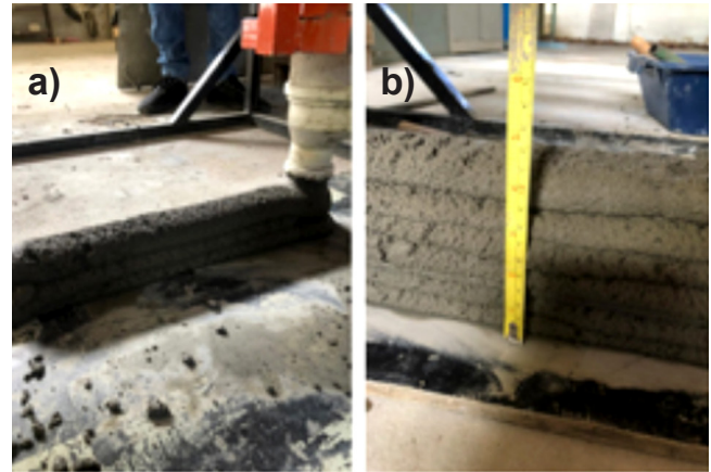
Figure 3: a) and b) Definition of the optimum water to dry material ratio for the printing conditions, reference mixture (1:2).
