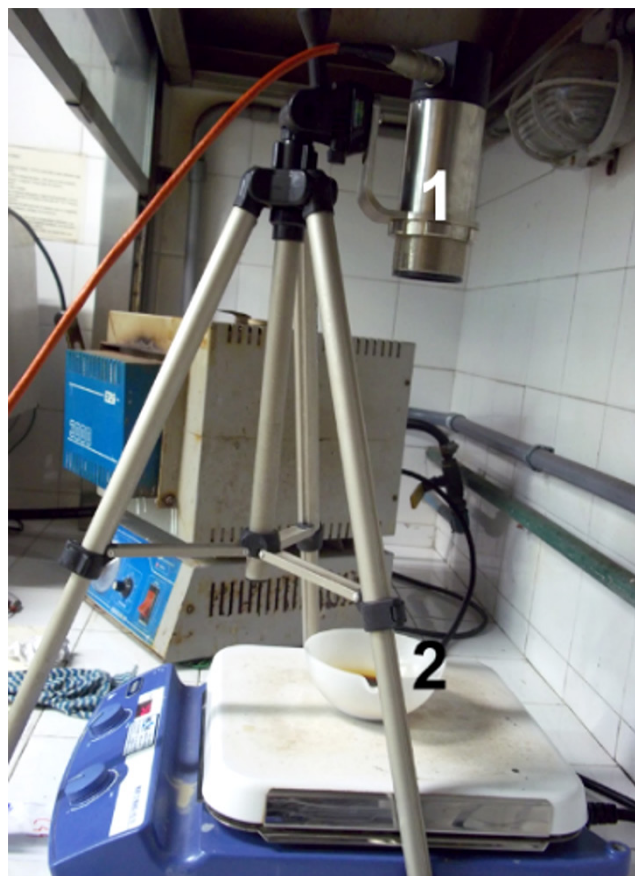
Figure 1: Temperature measurement during pyrolytic decomposition reactions of the dry gel: 1) pyrometer; and 2) sample.
