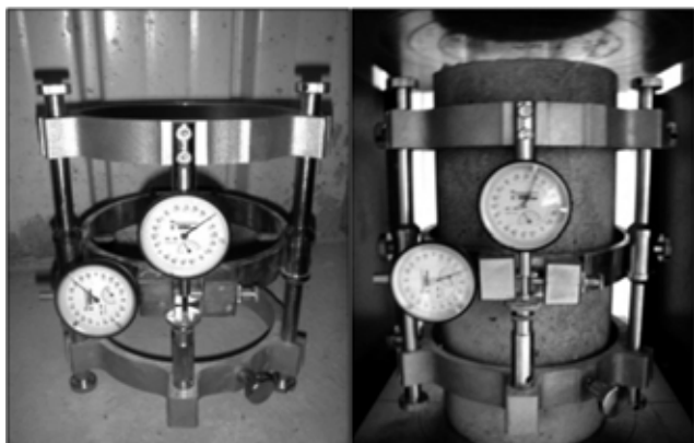
Figure 6: (a) Extensometer, (b) cylindrical specimen 16 cm x 32 cm before testing.
