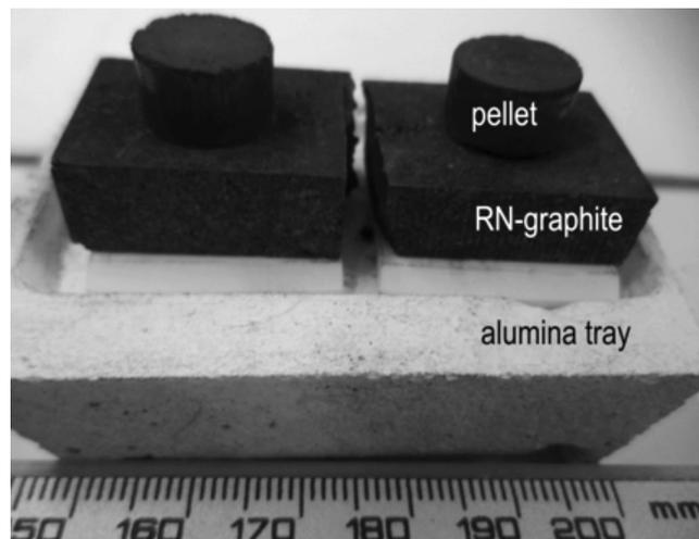
Figure 3: Wettability tests specimen setup.
