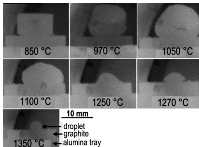
Figure 6: Wettability of RN graphite by Matte-A (850 °C to 1350 °C).
