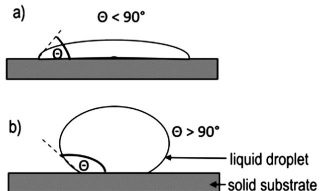
Figure 1: Schematic illustration of the sessile drop configuration (a) contact angle  $< 90^\circ$  (wetting system), (b) contact angle  $> 90^\circ$  (non-wetting system) [5].
