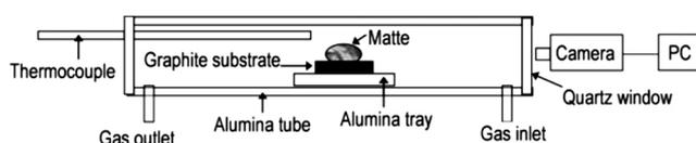
Figure 2: Schematic diagram of the CAF furnace setup.
