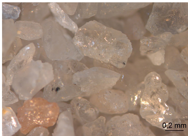
Figure 1: Image of AGC particles retained in the ABNT 200 mesh sieve, showing quartz particles with a vitreous shine.
