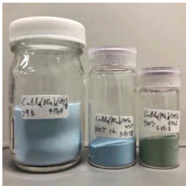
Figure 3 Photographs of samples heated at various temperatures, (a) without heating, (b) 500 °C, (c) 700 °C.
