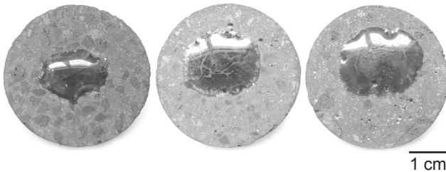
Figure 9: Samples showing the different liquid spreading on 10 SBC castables.
