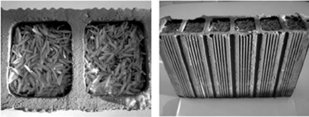
Figure 3: Hollow clay brick with agglomerated rice husk inside it (acoustic hollow clay brick).
