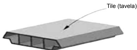
Figure 1: Conventional hollow clay brick. [Figura 1: Tabela convencional.]
