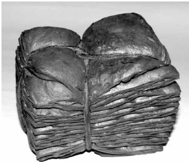
Figure 11: Assemblage of iron wire and pyro-expanded black slate fired up to 1220 °C; dimensions 14 cm x 12 cm x 9 cm.
