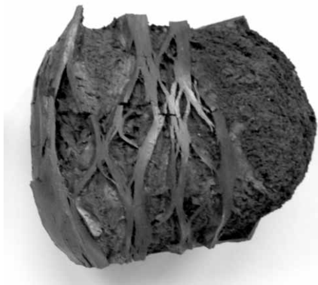
Figure 7: Black slate fired up to 1240 °C; dimensions 12 cm x 10 cm x 8.5 cm.
