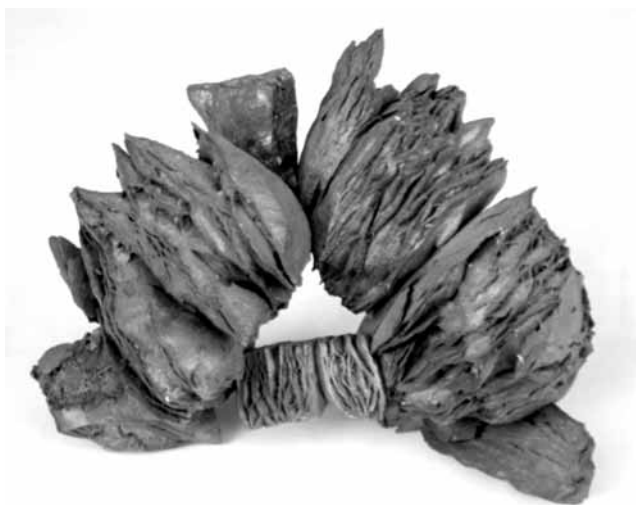
Figure 8: Pyro-expanded black slate fired up to 1160 °C; dimensions 19 cm x 15 cm x 15 cm.
