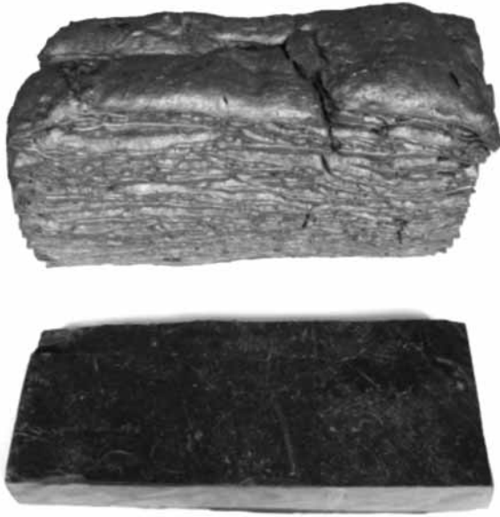
Figure 1: Black slate piece at room temperature (A) with dimensions 21 cm x 13.5 cm x 3 cm and after pyroplastic expansion up to 1200 °C (B) with dimensions 22 cm x 13.5 cm x 12 cm.
