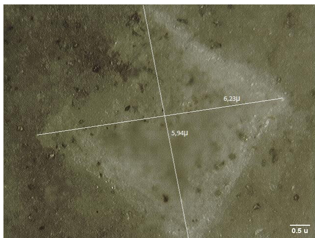
Figure 1: Image showing a discontinuity generated on the surface of the \text{Al}_2\text{O}_3/\text{SiC} ceramic sample.
