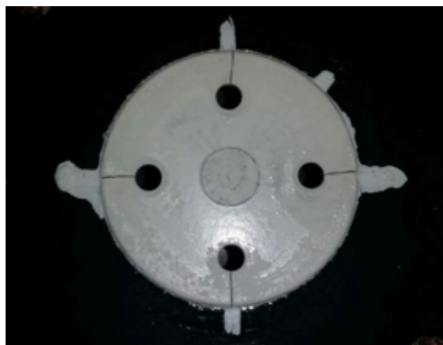
Figure 1: Welding lines in a ceramic part produced by LPIM process.
