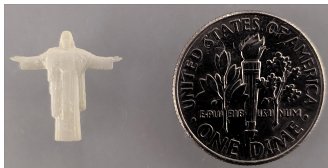
Figure 12: Zirconia part fabricated by vat photopolymerization [174].
