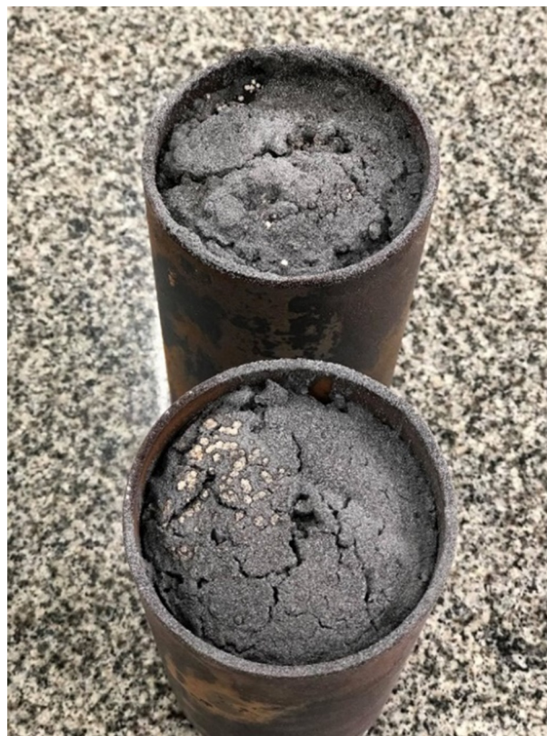
Figure 1: Image of RHA+NaOH after calcination at 750 °C for 2 h.
