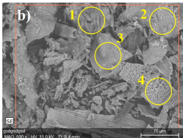
Figure 5: SEM micrographs showing areas selected for EDS analysis: a) fly ash; and b) RHA.
