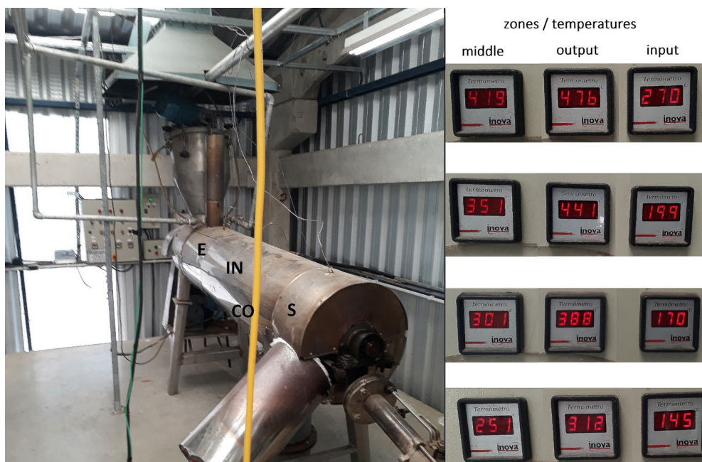
Figure 3: Pyrolysis reactor - screw conveyor type (Pyrolysis of biomass/waste) and temperature displays.
