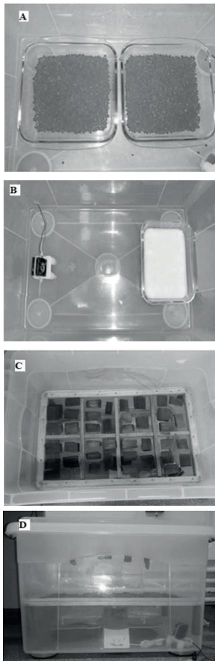
**FIGURE 1** Plastic box with silica gel (A); plastic box with K<sub>2</sub>SO<sub>4</sub> with a fan indoor air circulation (B); charcoal packaging (C) and set up test containing a saline solution, gauge of temperature and RH, fan and charcoal samples (D).
