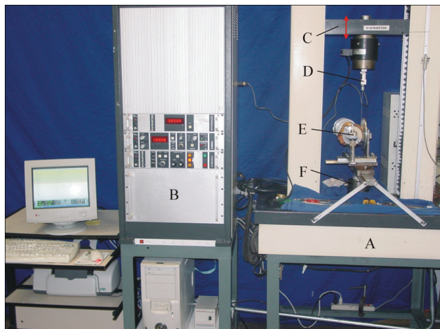
Figure 3 - KRATOS® testing machine used for the biomechanical study. A. Mechanical testing device. B. Data acquisition system. C. Testing machine pivo (arrow indicates direction of movement). D. Load cell (100 kgf). E. Knee fixed to the device. F. Base image of the knee fixed to the device.
