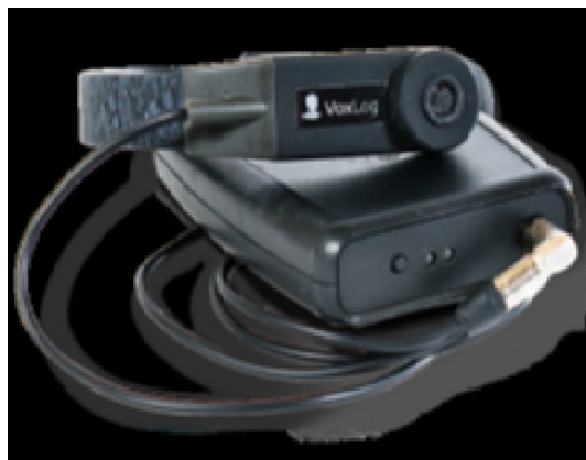
Source: http://www.sonvox.com/VoxLog_technical_document.pdf Figure 1. VoxLog® brand dosimeter from Sonvox model 3.1
