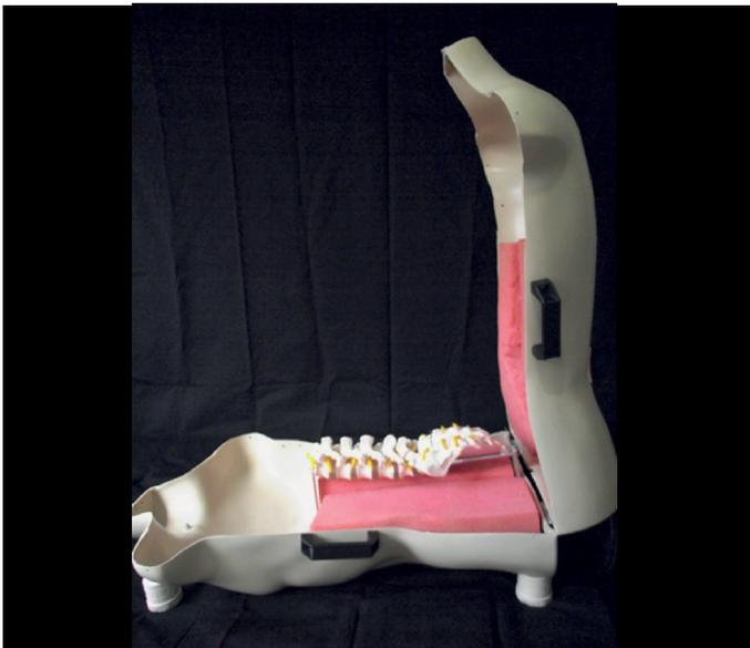
Figure 4. View of the internal space of the mannequin filled with the foam.
