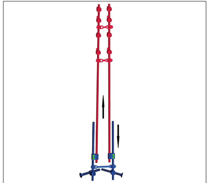
Figure 2. The bipolar telescopic construct.
