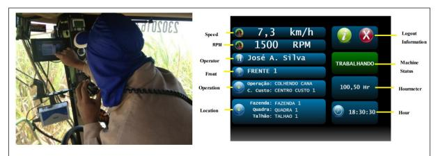
Figure 2 - Worker using the onboard management interface via onboard computer and screen of this interface with information such as speed, rotation, machine's working status, among others. Source: MANZONI (2015).
