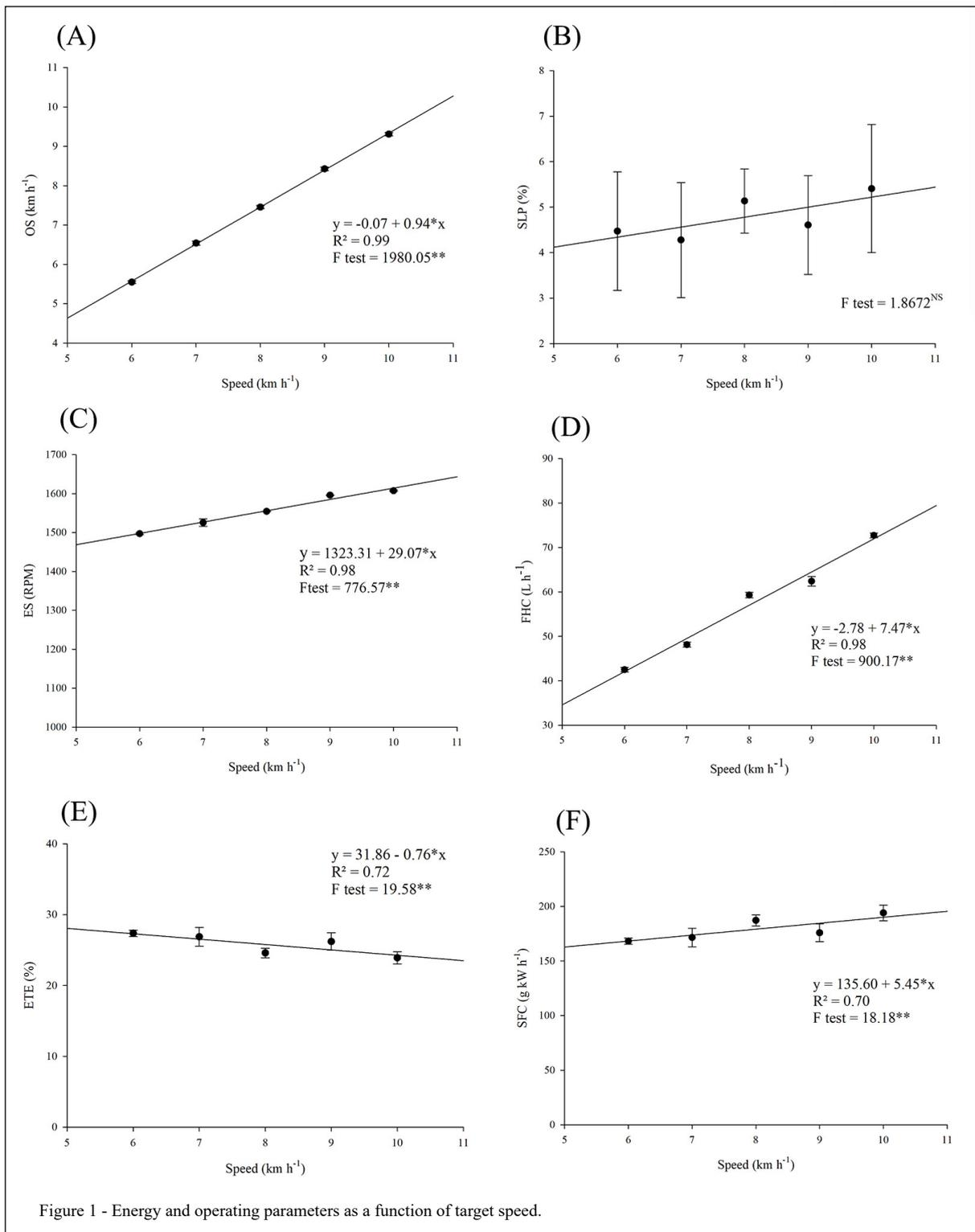
Figure 1 - Energy and operating parameters as a function of target speed.
