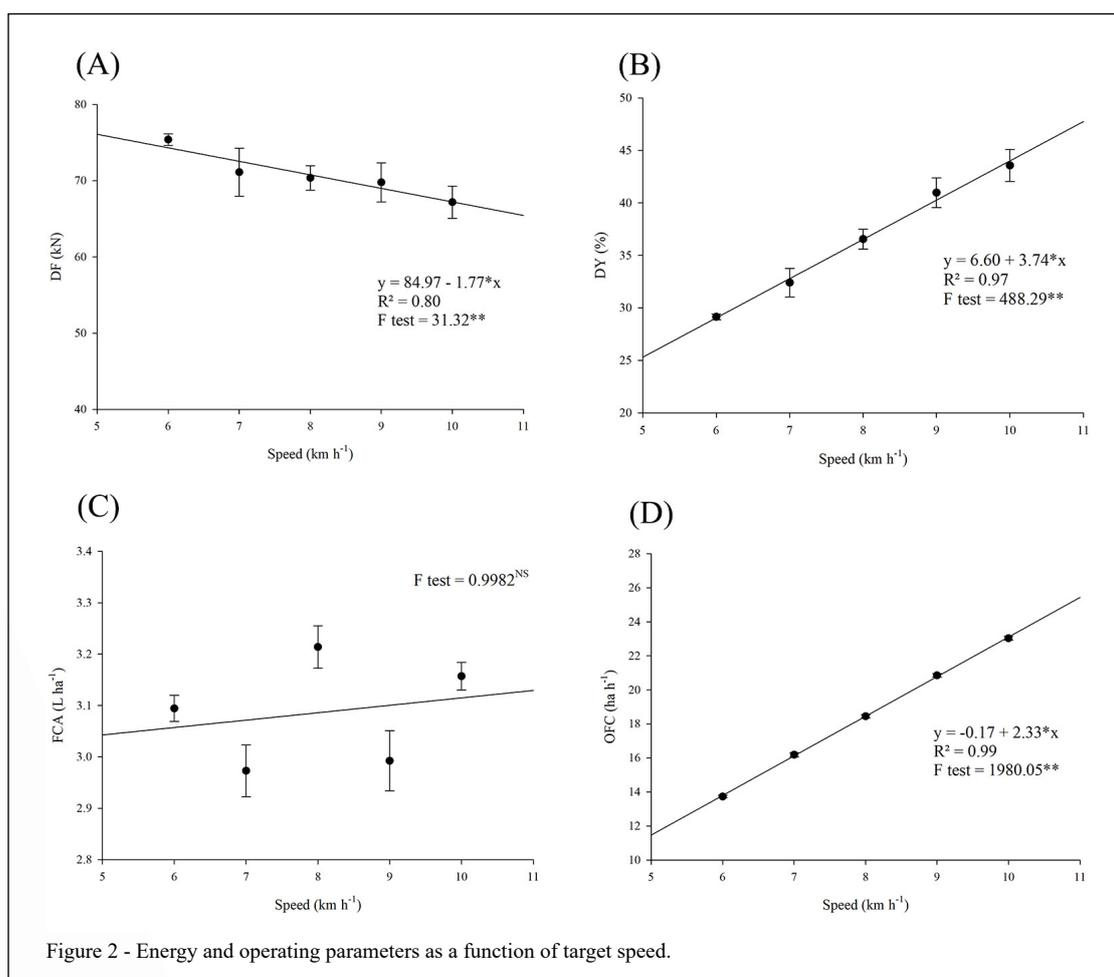
Figure 2 - Energy and operating parameters as a function of target speed.
