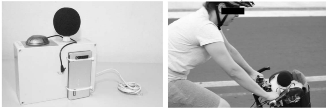
Figure 2. Noise sensor (left) and its position in the bicycle (right) used for data collection campaigns in the city of São Carlos-SP.
