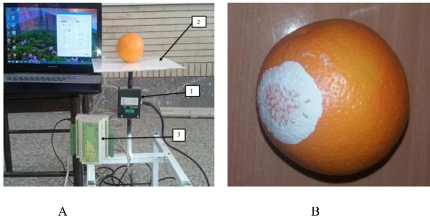
**Figure 11.** (A) Experimental dropping test setup. (1) Axial load cell, (2) rigid plate connected to the load cell, and (3) transmitter; (B) Determination of contact area for Stress calculation after impact.
