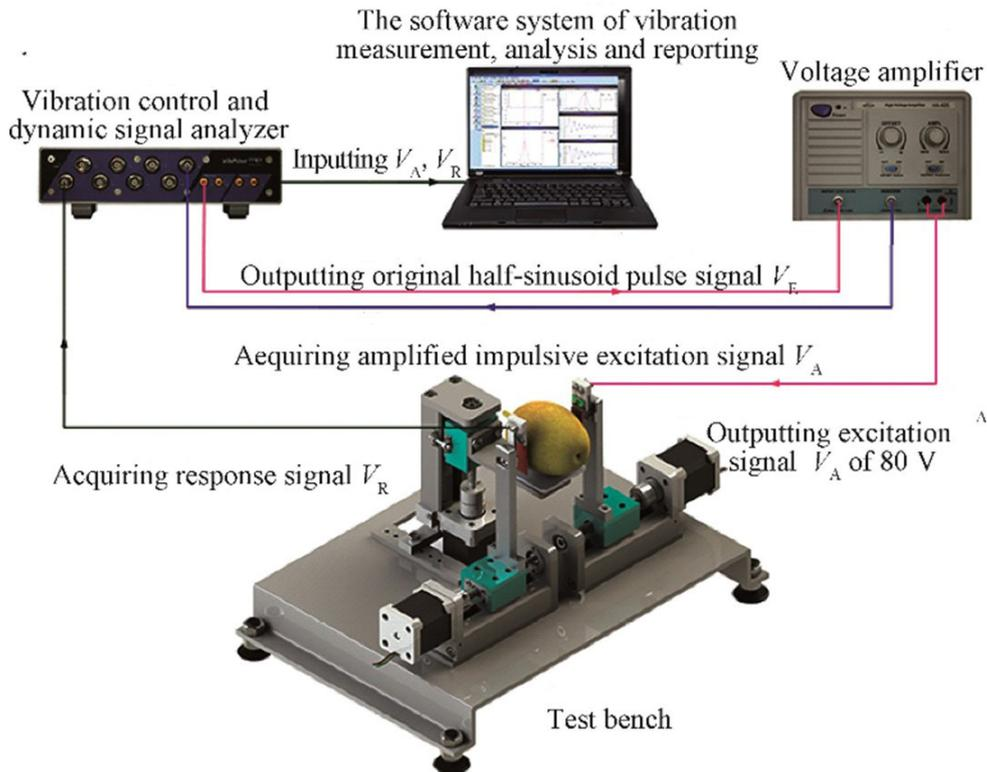
Figure 17. Pear acoustic vibration non-destructive testing system.
