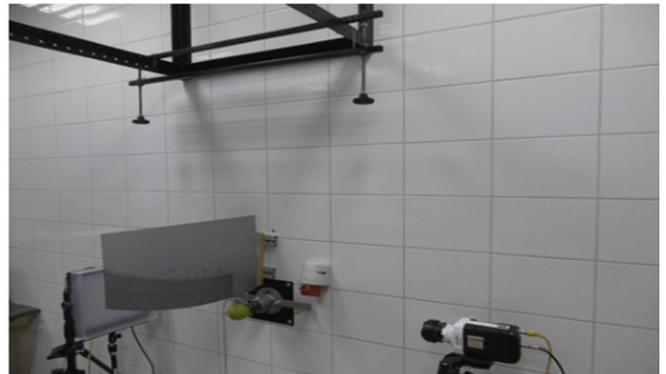
**Figure 9.** Impact test bench.
