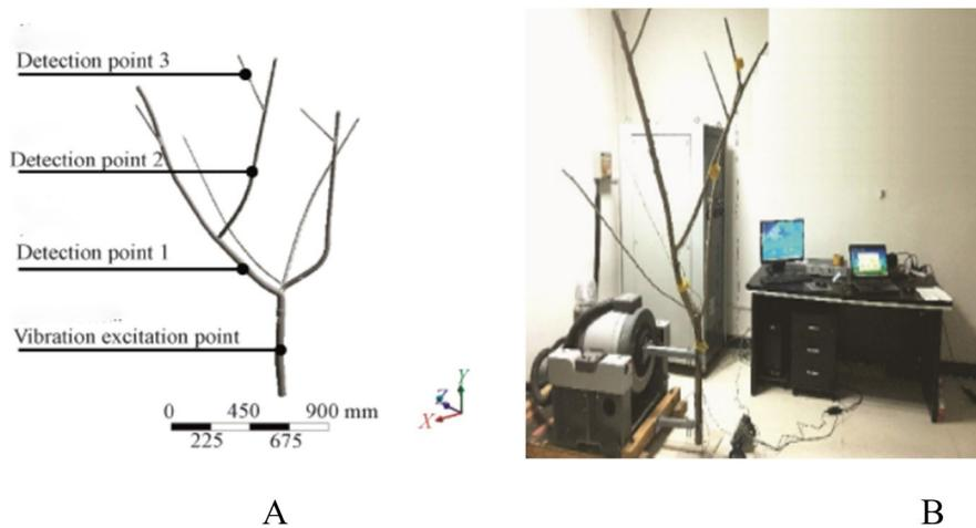
**Figure 6.** Almond finite element model (A) and vibration detection platform (B).
