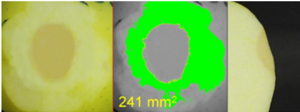
**Figure 8.** Comparison of fruit surface and bruise depth images.
