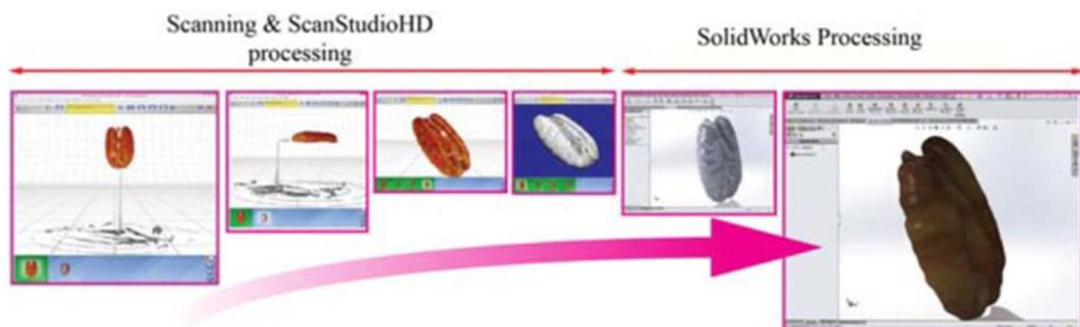
Figure 13. Walnut fruit digitization and finite element modeling process.
