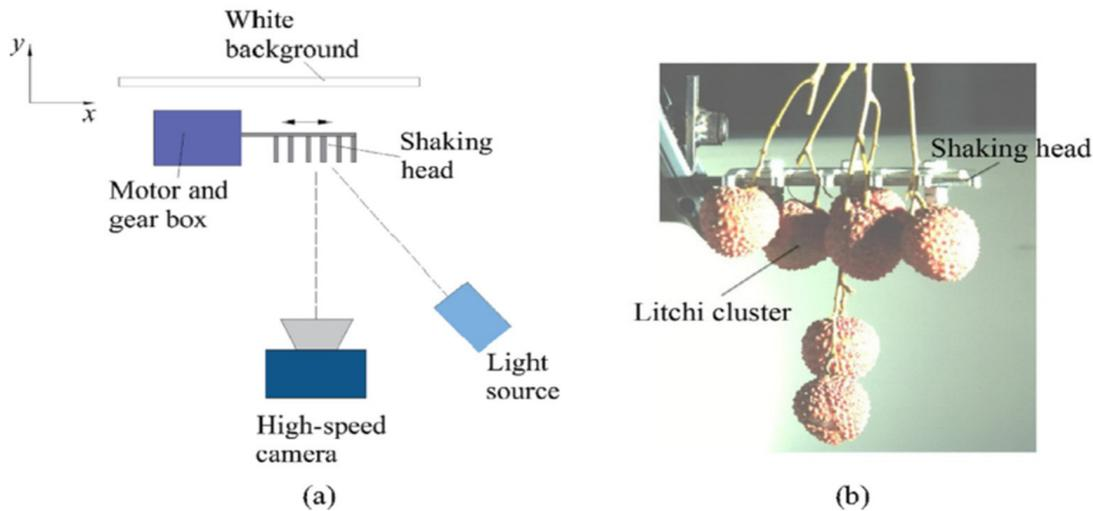
Figure 3. (a) Schematic diagram of vibration detection device; (b) Moving image of litchi captured by high-speed camera.
