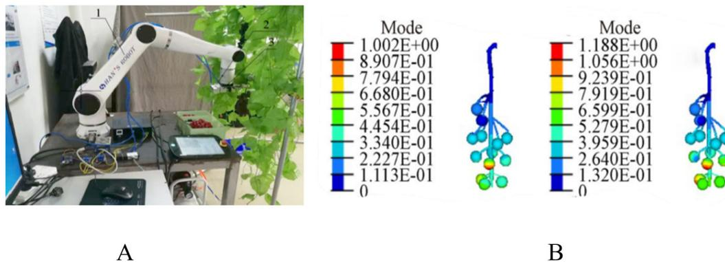
Figure 4. (A) The picking test bed; (B) modal analysis of grape bunches (order 4 ~ 5).
