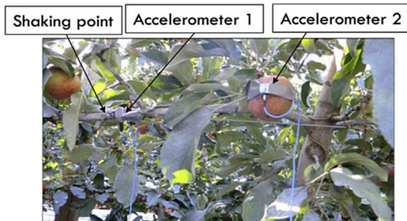
**Figure 10.** Position of shaking point and installed sensors.
