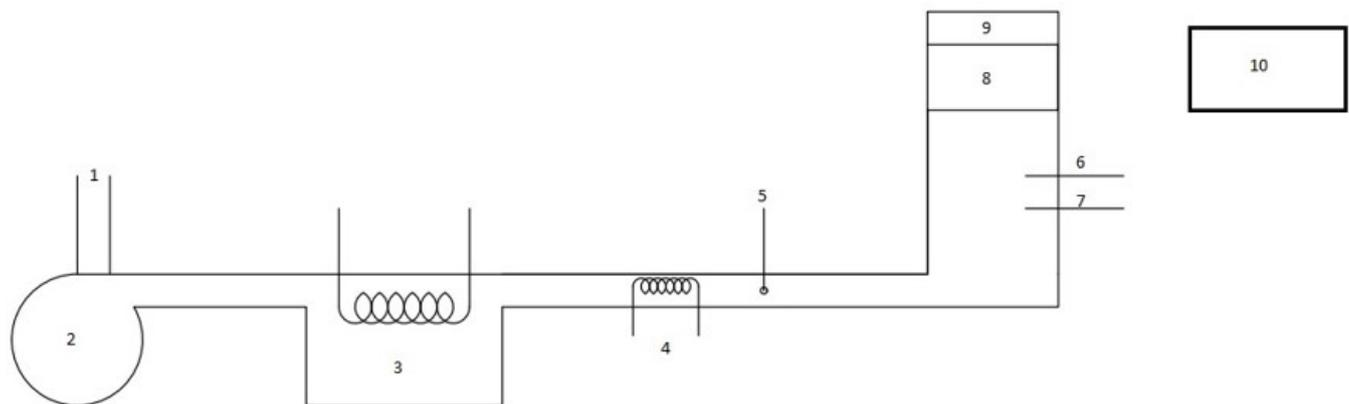
**Figure 2.** Schematic of the drying equipment. 1 = air entrance; 2 = blower; 3 = condenser; 4 = resistors; 5 = vapor injector; 6 = velocity sensor; 7 = air temperature and relative humidity sensor; 8 = drying chamber; 9 = load cell; 10 = PLC: Programmable Logic Controller.
