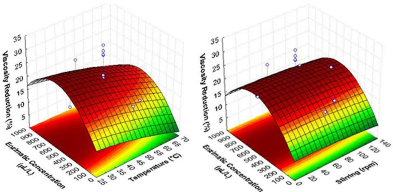
**Figure 4.** Response surface and response profile for viscosity reduction of free pectinase as a function of temperature and enzyme concentration and enzyme concentration and stirring.
