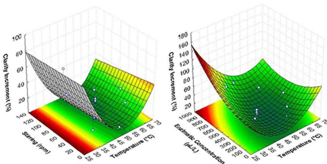
**Figure 1.** Response surface for the clarity increment for the enzyme as a function of temperature and enzymatic concentration and enzymatic concentration and stirring.
