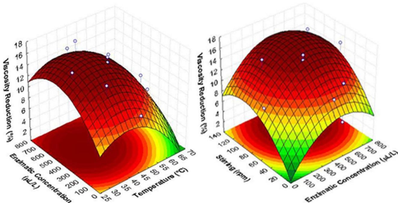
**Figure 3.** Response surface and response profile for the viscosity reduction of free pectinase as a function of temperature and enzymatic concentration and temperature and stirring.
