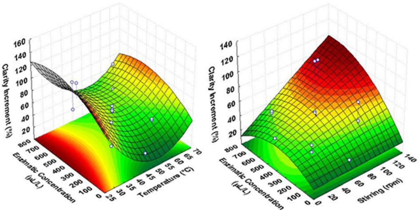
**Figure 2.** Response surface and response profile for the clarity increment of the encapsulated enzyme as a function of the temperature and stirring and temperature and enzymatic concentration.
