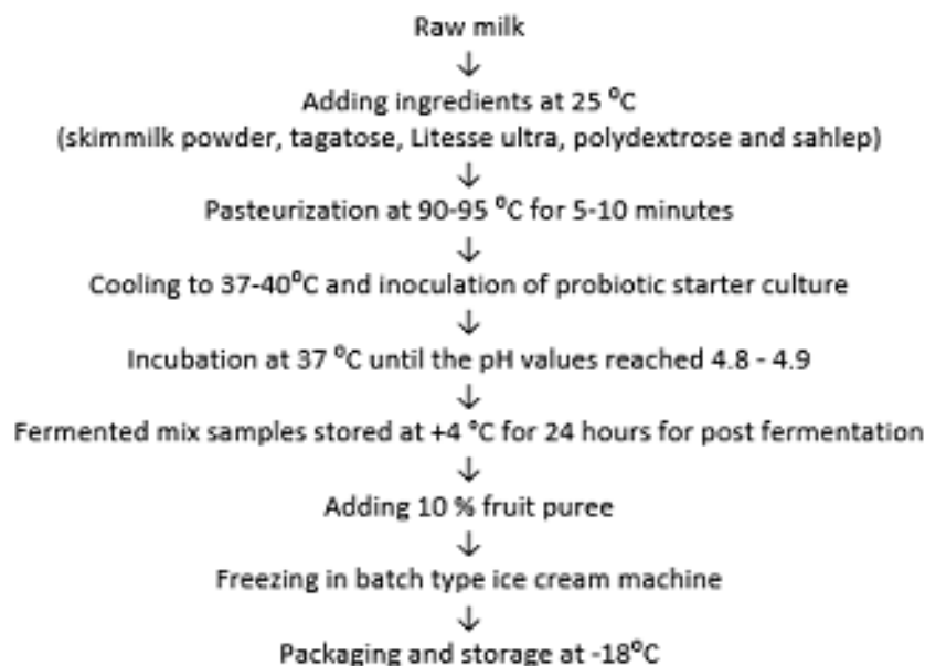
Figure 1. Flow diagram of synbiotic ice cream with fruit puree.
