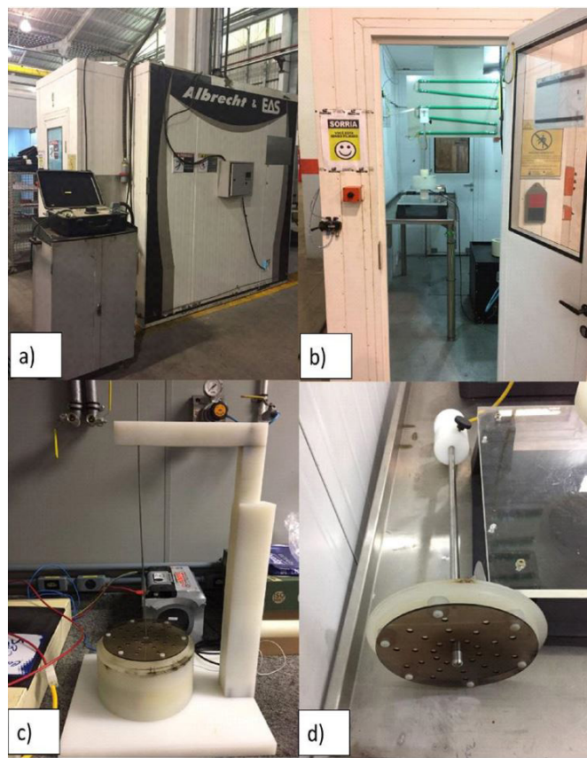
Figure 1. Electro-neutralizer apparatus. Legend: a) External view; b) chamber internal view; c) sample holder; d) electro-neutralizer device in detail (spark generator).
