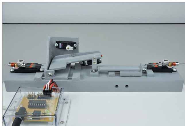
Figure 2 - Experiment device configuration. Note the four servo motors at the end of the gray support and the controlling plate for the computer interface.
