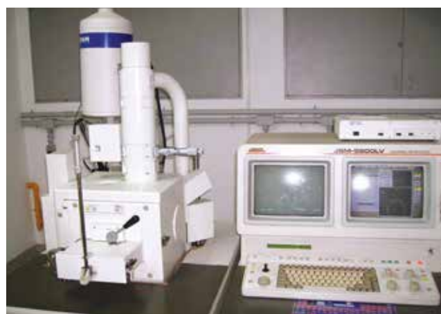
Figure 1 - Scanning electronic microscope used with EDS system of microanalysis.
