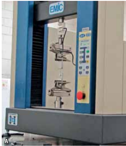
FIGURE 2 - A) EMIC Universal Testing Machine and B) testing device.
