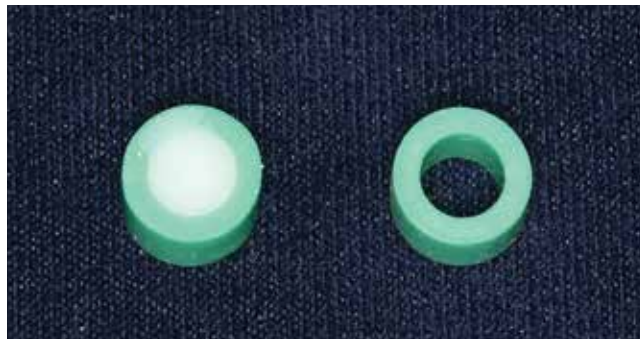
Figure 1 - Silicone molds used to fabricate the test specimens.
