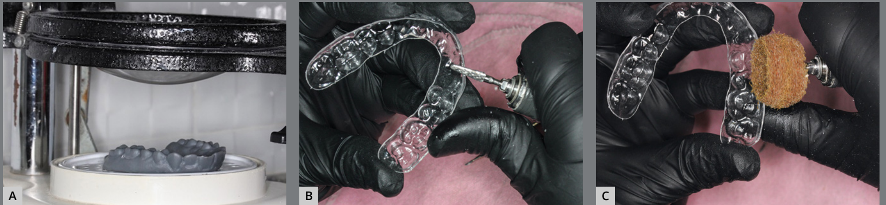
Figure 17: Digital workflow for manufacturing of thermoformed retainer appliance: A) thermoforming; B) finishing and C) polishing.
