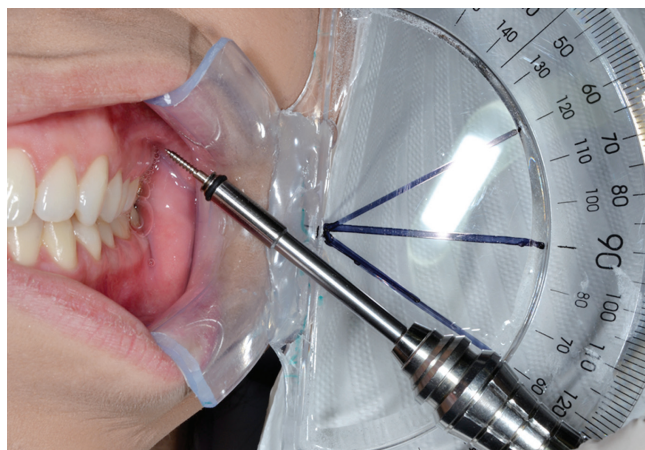
Figure 1 - The manual driver tip positioned beside the flat surface of the protractor over the 60° angle.
