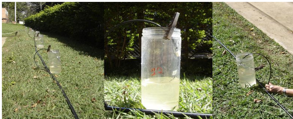
FIGURE. 2. Field experiment of the microsprinkler with microtube.
