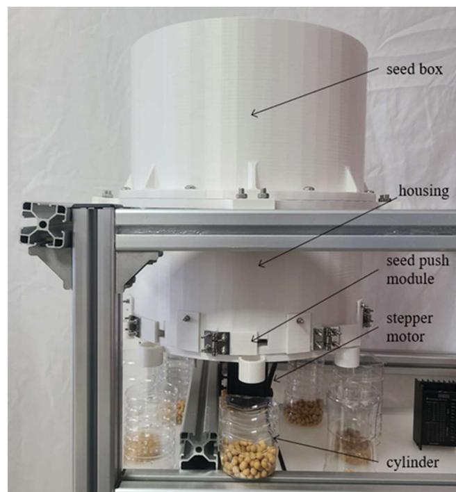
FIGURE 15. Setup used for the benchtop validation test
