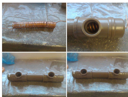
d) Shell-tube condenser
