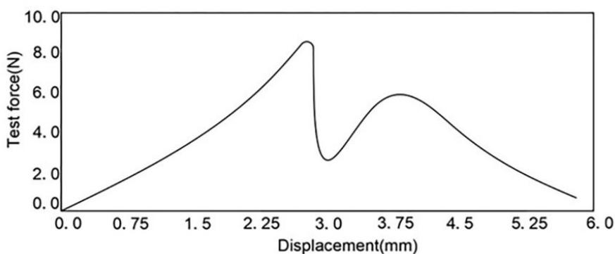
FIGURE 14. Shear load curve of watercress stem.
