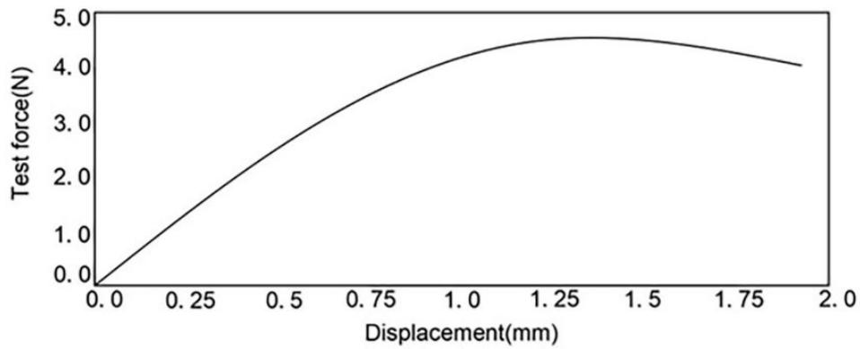
FIGURE 9. Radial compression load curve.
