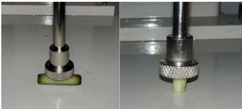
FIGURE 3. Watercress compression test process.
