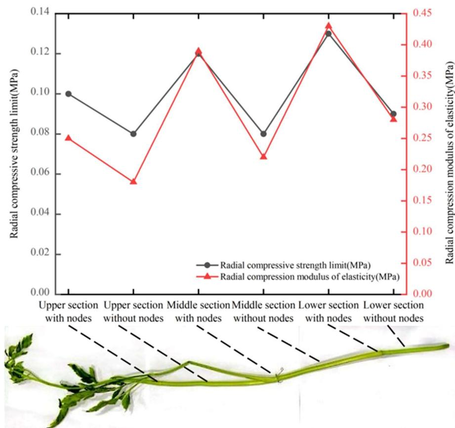
FIGURE 11. Curves of radial compressive strength and modulus of the elasticity of the watercress stalks as a function of the sampling portion.
