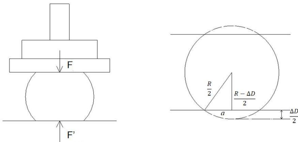
FIGURE 10. Experimental diagram of radial compression of the watercress stalks.
