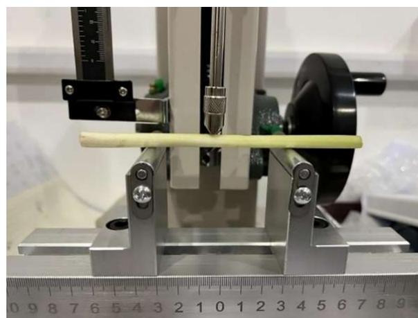
FIGURE 5. Watercress bending test process
