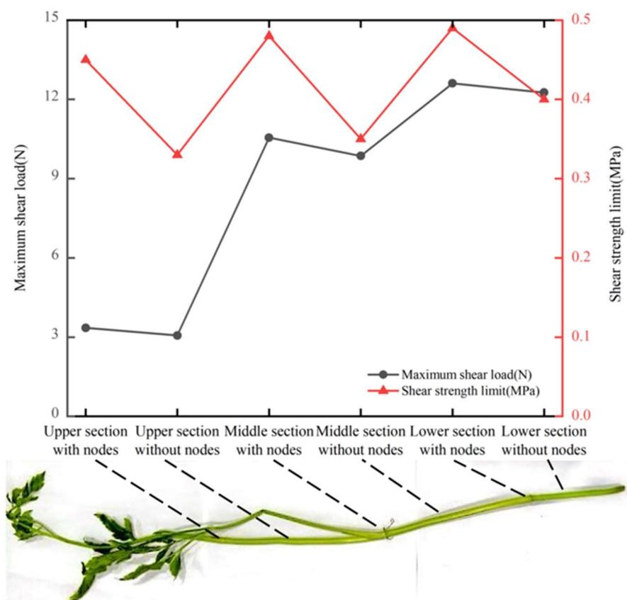
FIGURE 15. Curves of the shear load and modulus of the watercress stalks as a function of sampling location.
