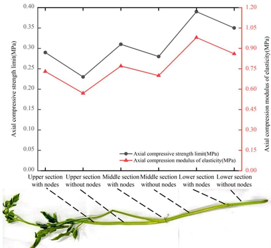
FIGURE 13. Curves of the axial compressive strength and modulus of the elasticity of the watercress stalks as a function of the sampling portion.
