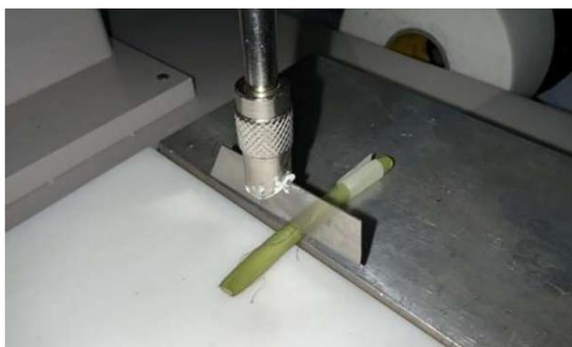
FIGURE 4. Watercress shearing test process.
