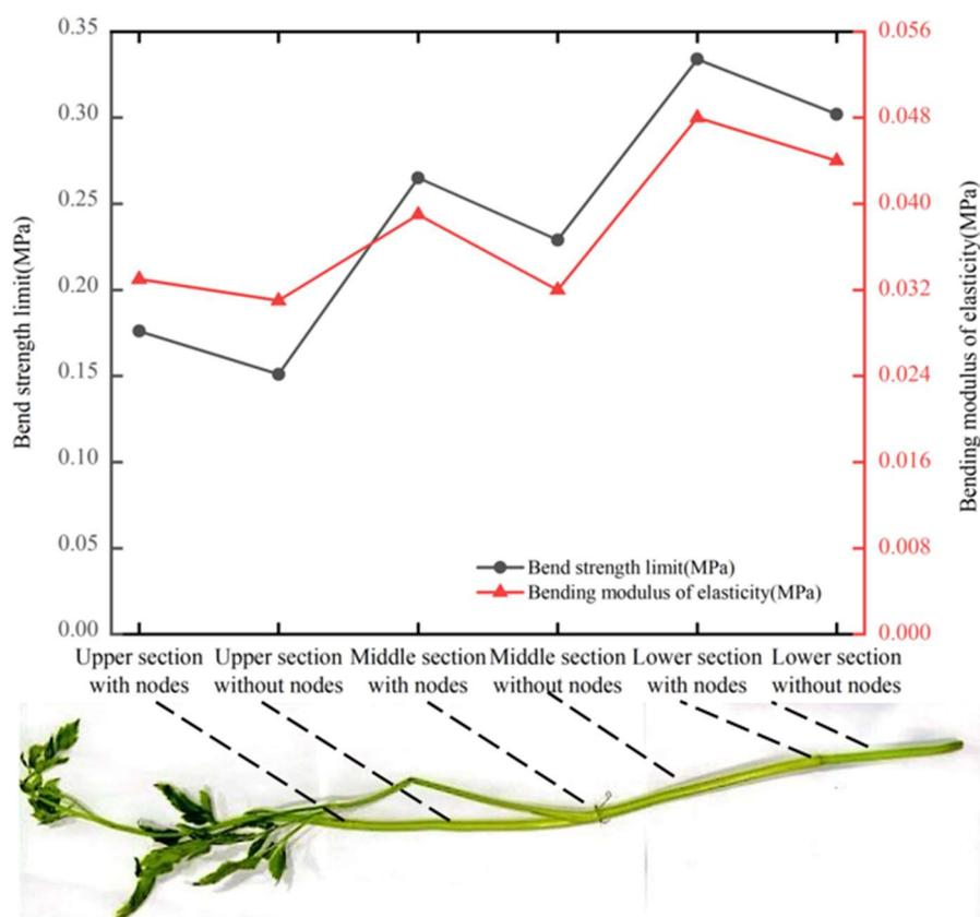
FIGURE 16. Curves of the flexural strength and modulus of the watercress stalks as a function of sampling location.
