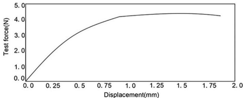
FIGURE 12. Axial compression load curve.
