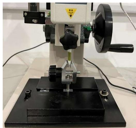
FIGURE 2. Watercress tensile test process.
