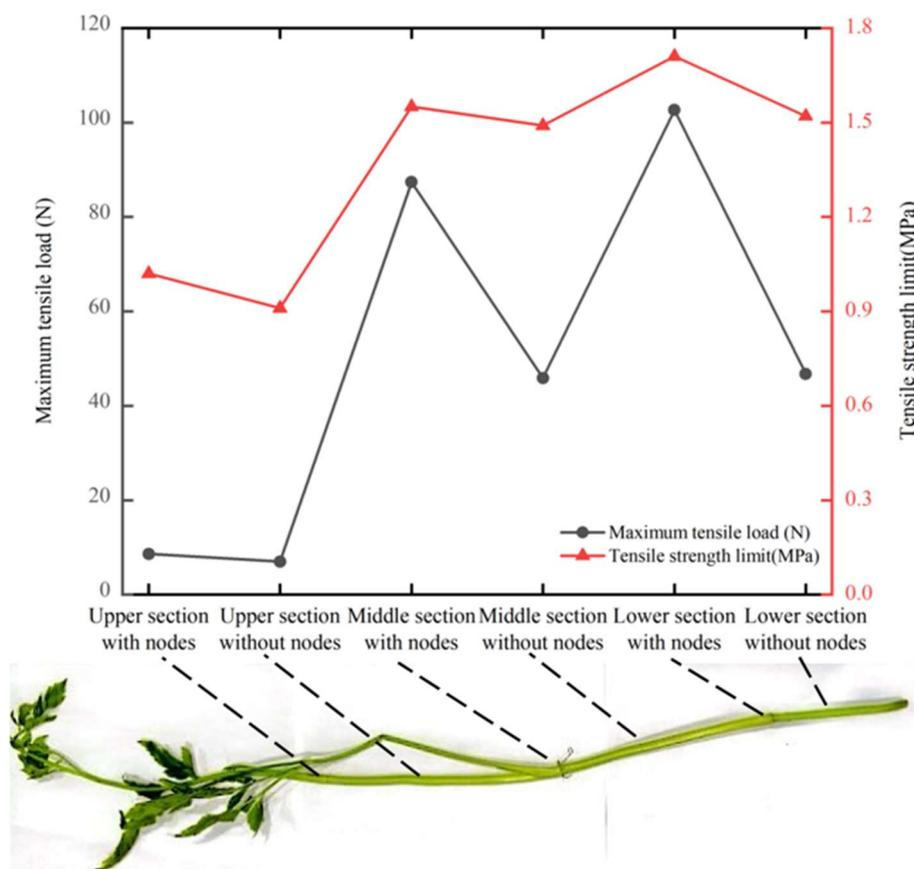
FIGURE 8. Curves of maximum tensile load and strength of the watercress stalks as a function of the sampling portion.
