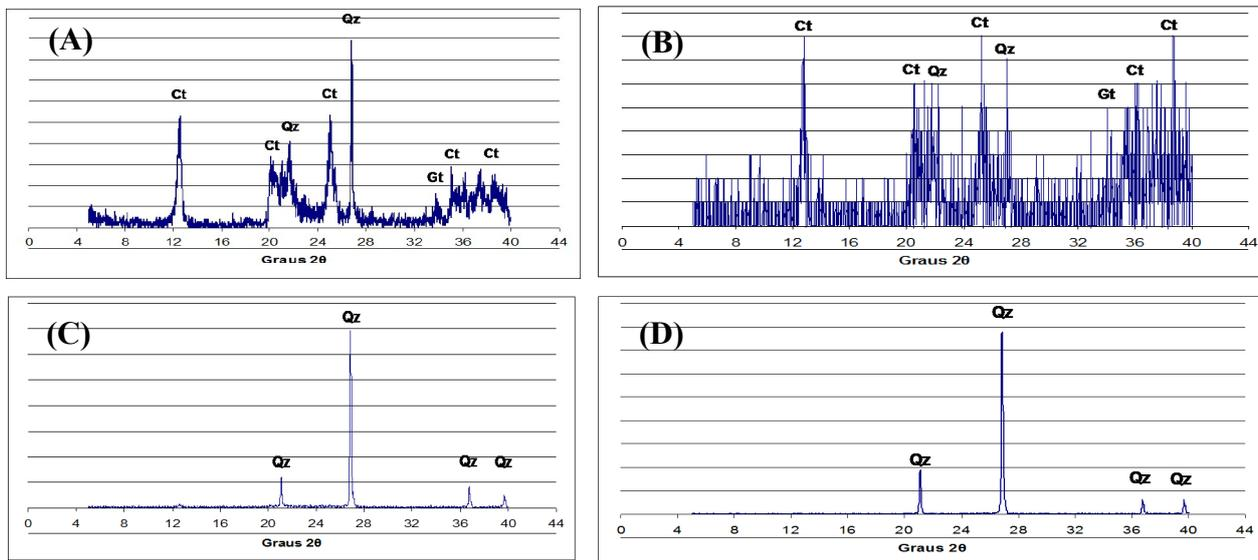
FIGURE 2. X-ray diffractograms - (A) silt and clay fractions of the Bt2 horizon of the Argissolo Amarelo (Humic Clayic Xanthic Acrisol); (B) silt and clay fractions of the Bt2 horizon of the Argissolo Vermelho Amarelo (Clayic Rhodic Acrisol); (C) silt and clay fractions of the A horizon of the Neossolo Quartzarênico (Hydrophobic Ochric Dystric Arenosol); (D) silt and clay fractions of the C2 horizon of the Neossolo Quartzarênico (Hydrophobic Ochric Dystric Arenosol).
