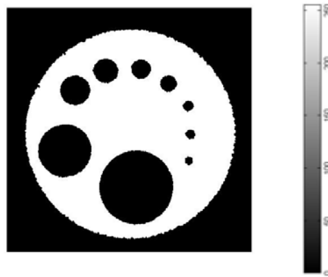
FIGURE 10. Image generated after setting the element in the disk shape and in the operation of opening and closing.
