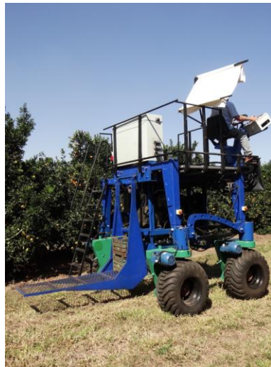
FIGURE 5. Mobile platform in harvest position with a picking station. (A) Front view. (B) Back view, showing narrow platform for box disposal.
