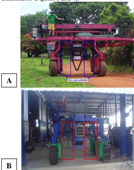
FIGURE 3. (A) Former mobile unit showing fixed gauge and a narrow gap for plant rows (on blue lines). (B) New prototype with retractable gauge and showing expanded space for plant rows (on red line).
