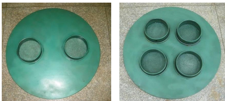
FIGURE 2. Drying bed in thin layer with two (left) and four (right) trays.
