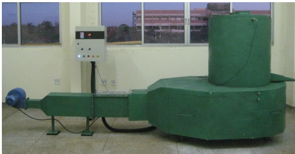
FIGURE 6. Experimental dryer for drying agricultural products in thin and thick layer.
