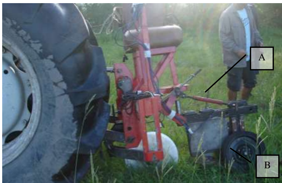
FIGURE 4. Tool bar frame with force measuring device and hoe set, where: (A) regulatory arm of the inclination of the hoe, and (B) wheel depth control.
