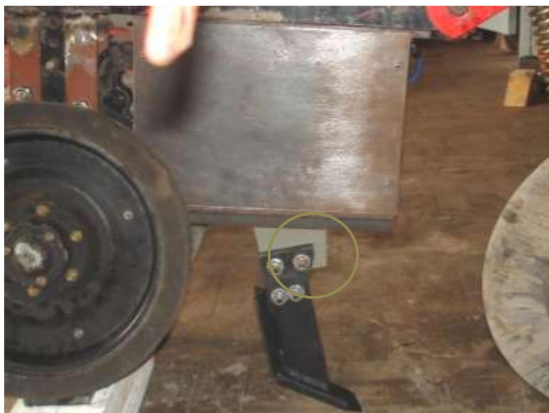
FIGURE 3. Force measuring device assembled in the row with the hoes attachment detail.
