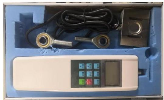
FIGURE 3. HF-5KN digital display push-pull gauge.
