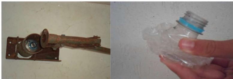
FIGURE 1. Equipment used to crush PET bottles and detail of the final condition of the bottle used as support material.
