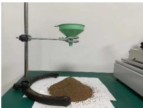
(a) Angle of repose test equipment
