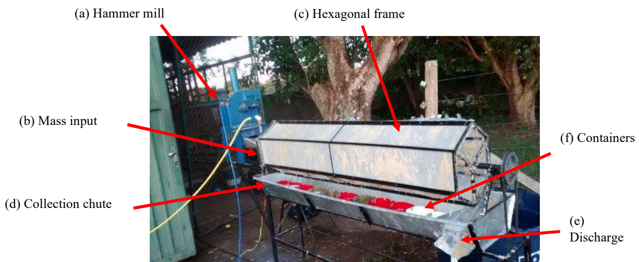
FIGURE 1. Hexagonal sieve for separating the starch-water suspension from the fibrous bagasse.
